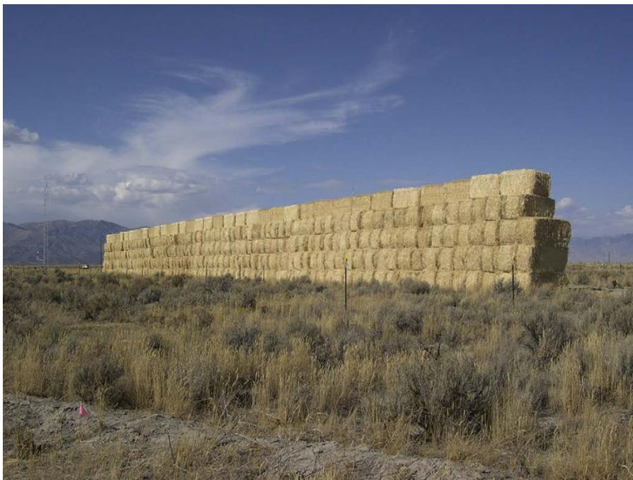
**Figure 16: Mock straw bale sound barrier, 6 m high and 90 m long. (Finn et al. 2010)**
