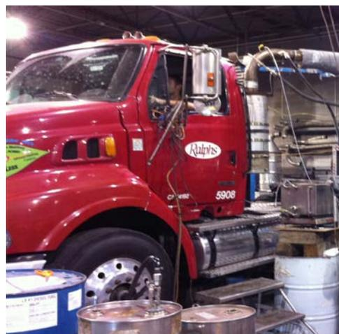
Figure 1. Test Vehicle during chassis dynamometer testing.
