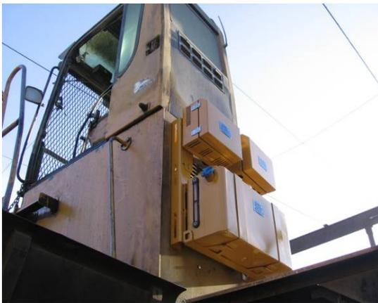
Figure 2. DPF/SCR Components on Excavator
