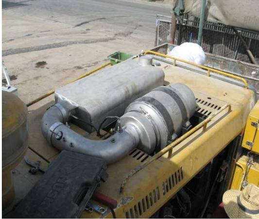
Figure 1. DPF and SCR Catalyst on Loader
