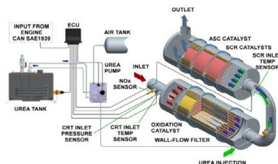
The CRT was previously verified by ARB as a level 3 PM control device (>85% reduction) that also meets the 20% NO<sub>2</sub> requirement for 1998-2002 MY heavy duty diesel engines. The SCR system uses NH<sub>3</sub>, carried on the vehicle as urea, to reduce NO<sub>x</sub> over a vanadium based catalyst. The precise air assisted injection of urea is performed using an OE dosing pump controlled by an ECU that was developed by JM.
