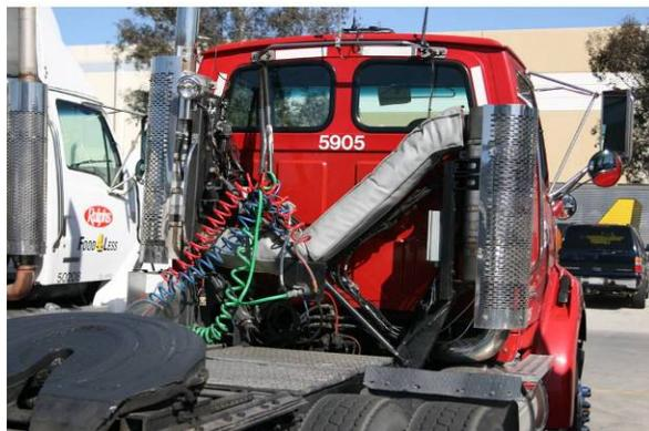
Figure 15: Truck Equipped with SCRT™
