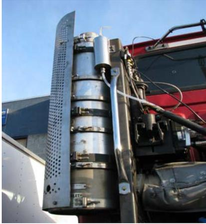
Figure 2. SCRT system installed on the test vehicle.
