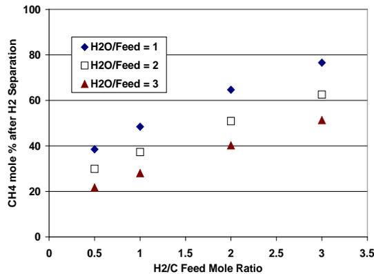
**Figure 3.** Methane concentration in final product gas. It can be seen that the final product gas contains significant quantities of methane, which is up to ~80 molar %, or up to ~90 mass % at the optimum process condition, which is 1:1 ratio of water to feedstock mass ratio.
