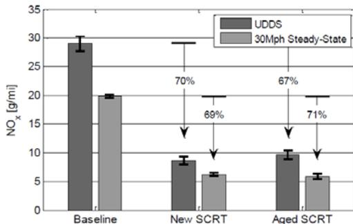
Figure 3. Results of NO<sub>x</sub> emissions from baseline, new SCRT and aged SCRT configurations.
