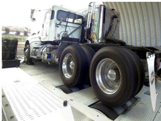
**Figure 5: WVU Transportable Chassis Dynamometer**
