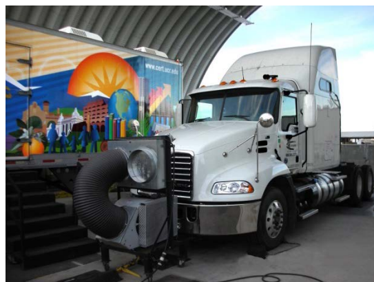
Figure 1: Truck being tested on chassis dynamometer
