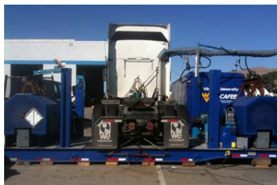
Figure 1: Test Vehicle during chassis dynamometer testing
