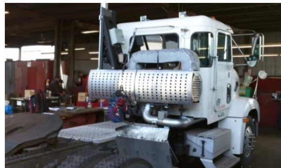
Figure 2: SCRT Typical System Installation
