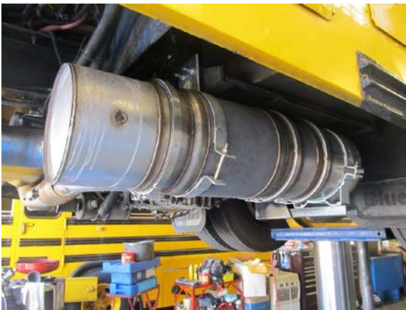
Figure 2: Donaldson LNF installed on Bus 55
