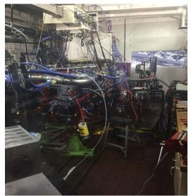
Figure 1: Test Engine on Dynamometer
