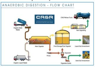
Figure 15: CR&R's Anaerobic Digestion Flow Chart
