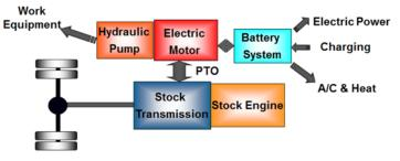
Figure 37: Odyne Plug In Hybrid System
