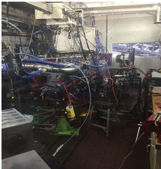
**Figure 1: Test Engine on Dynamometer**
