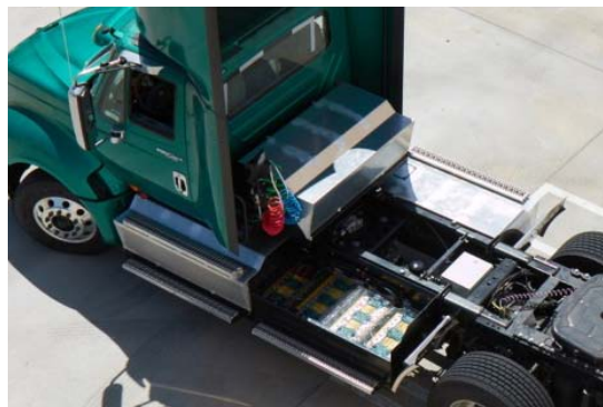
Figure 1: A demonstration vehicle equipped with Inverter-Charger Unit
