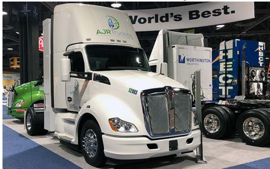
Figure 16: Class 8 Tractor with 12-Liter NG Engine
