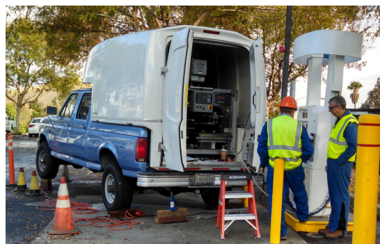
Figure 1: DMS staff testing a hydrogen dispenser
