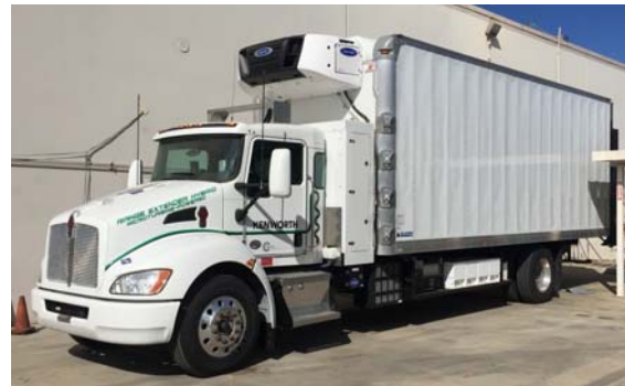
Figure 1: Hybrid Kenworth Class 7 Reefer truck with CNG powered Capstone turbine
