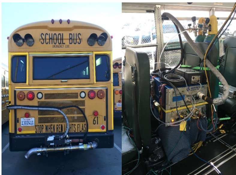
Figure 4: PEMS Equipment Install on School Bus
