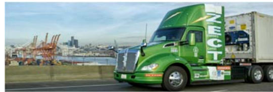
Figure 1: Zero Emission Electric Drayage Truck with Fuel Cell Range Extender
