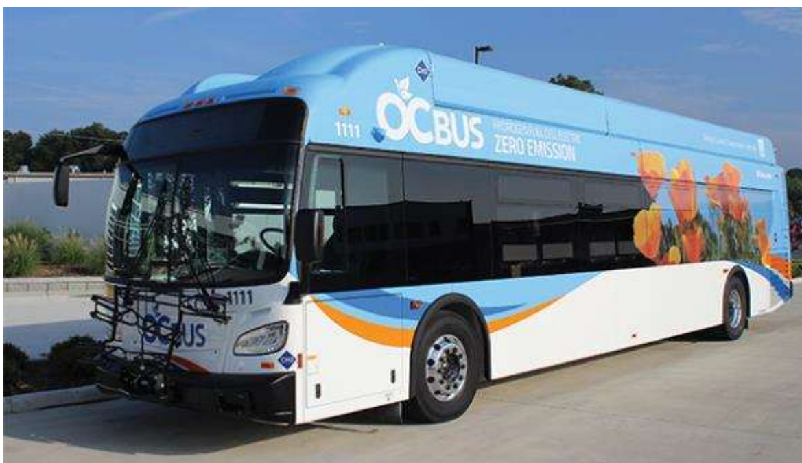
Figure 25: New Flyer XHE60 Xcelsior Fuel Cell Bus Deployed at OCTA
