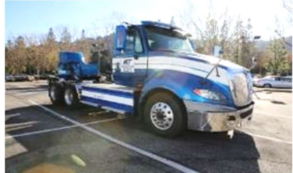
Figure 16: eTruck-2 with 280 kWh NMC 6-Pack
