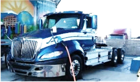
Figure 15: eTruck-1 with 180 kWh LFP 11-Pack
