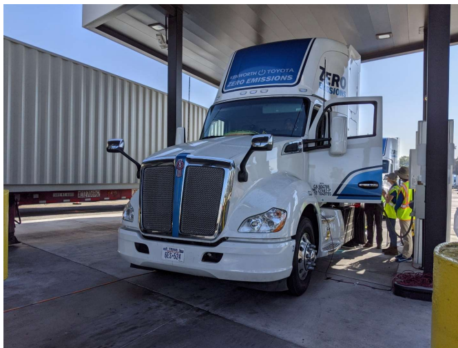
Figure 8: Kenworth – Toyota Class 8 FCET fueling at Shell Ontario Heavy-Duty Hydrogen station July 2021
