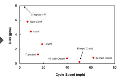
EMFAC2017 Example for NOx vs. Average Cycle Speed (Speed Correction Factor)
