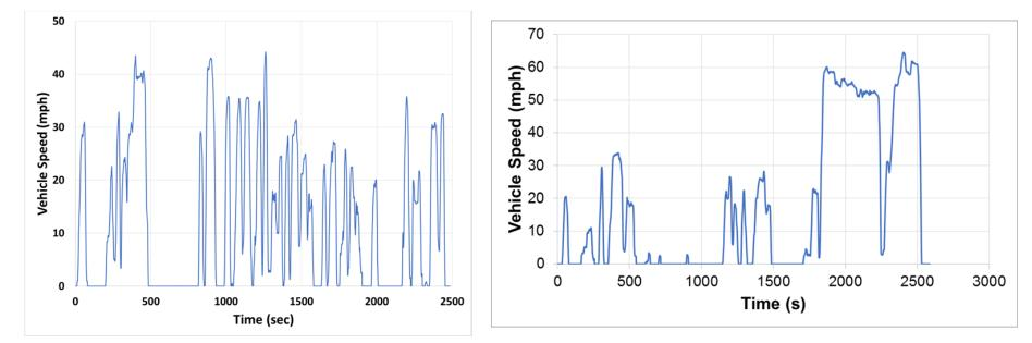
School bus cycle Ave. Speed: 12.3 mph / 19.68km/h Max. Speed: 45 mph / 72 km/h Delivery cycle Ave. Speed: 17.4 mph / 27.84km/h Max. Speed: 64 mph / 102.4 km/h
