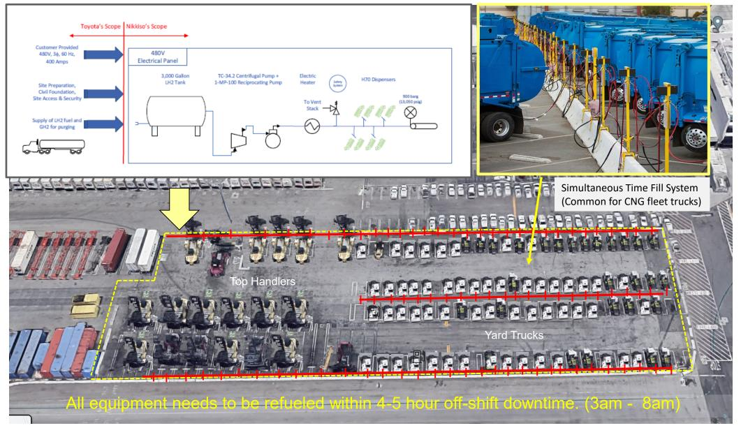
Together with hydrogen mobile refueler, this refueling system will support the hydrogen supply to port terminals 15
