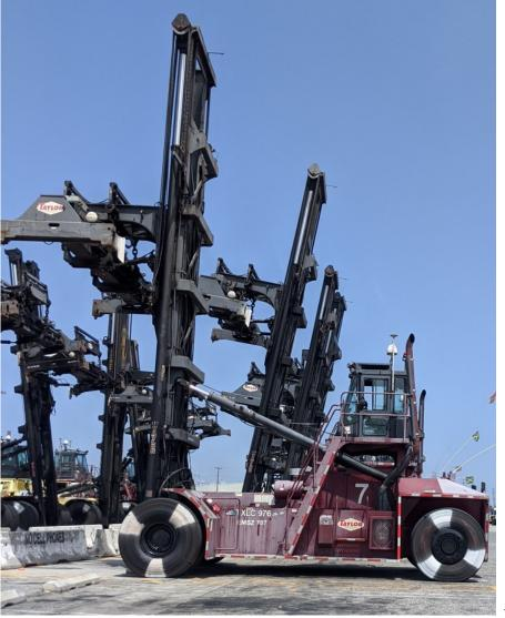
•FC Top Handler (Repower) FC:1 set : 80kW, (TMNA) => 2 sets 160kW •H2 Tank : 60kg@350bar => 122kg@700bar •Battery: 105kWh
