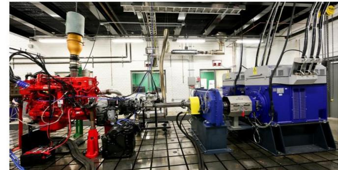
Figure 16. ISX450 engine and UltraShift Plus AMT under test in the Powertrain test cell of ORNL's VSI Laboratory.
