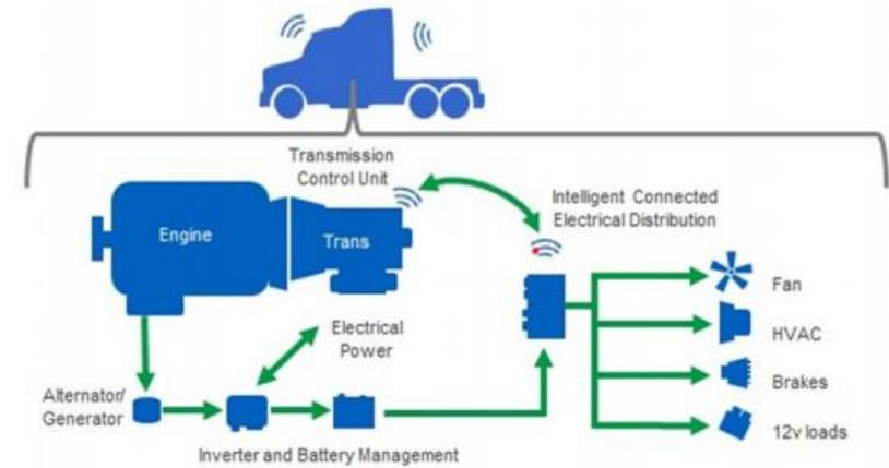
Figure 7. Schematic of a 48-volt commercial vehicle.
