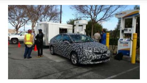
Hydrogen Fueling protocol J2601 testing with HySTEP equipment (trailer)
