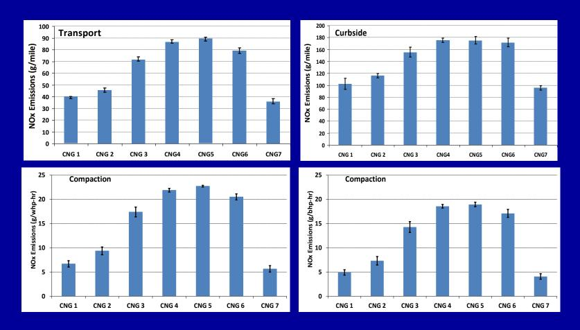
Refuse truck showed the strongest fuel effects compared to the three buses, especially for the compaction segment with NOx increase of 286% over CNG 1.
