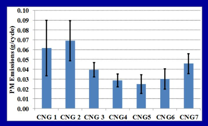
Richer gases with more higher hydrocarbons showing lower PM levels, while the gases with higher MN showed higher PM levels.
