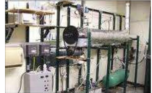
Figure 7 Kiln Steam Hydrogasification Reactor
