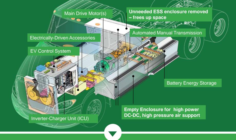
Base vehicle component layout easily accepts range extending technologies
