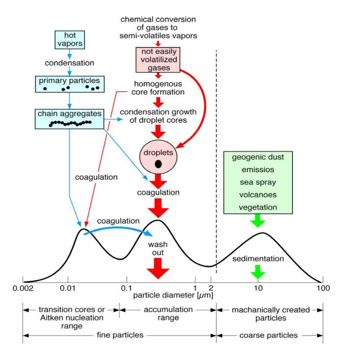
Formation of fine and ultrafine Particles: 2 different Mechanismes
