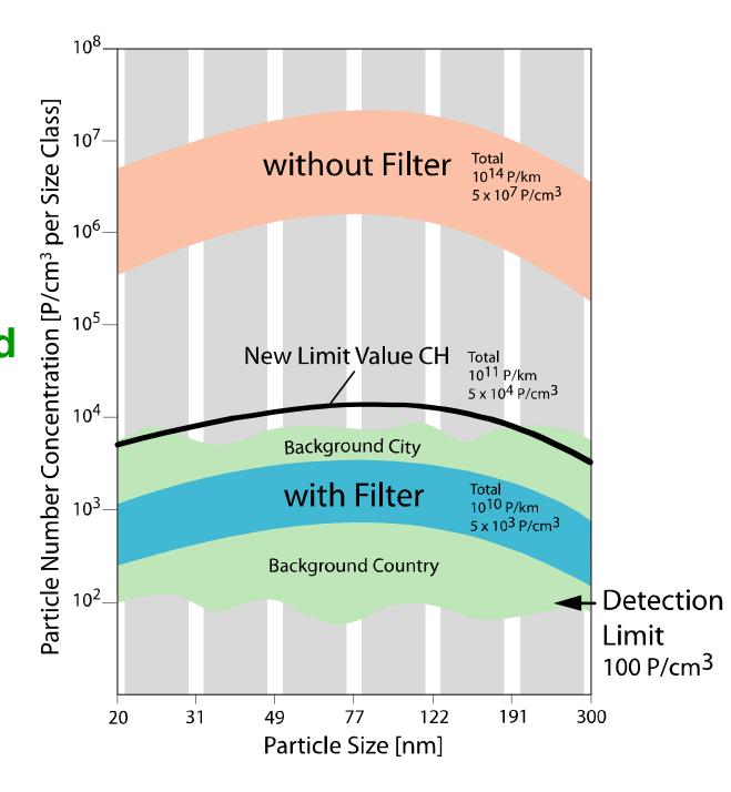
address the HE-metric and force the introduction of best available Technology Exhaust Gas downstream of the Filter is cleaner than Ambient Air !
