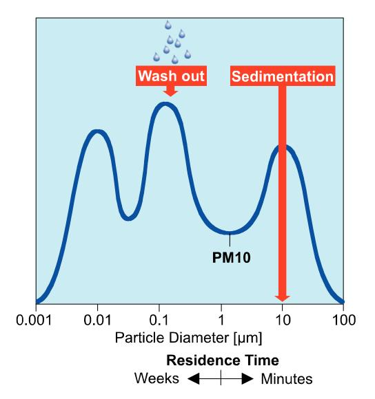
IC-Engine-emitted solid Nanoparticles a Part of PM10 but the most critical Fraction
