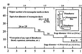
Duct Diameters Downstream from Flow Disturbance\* (Distanc
