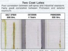
Acrylic Latex Primer/Topcoat System; PVC 34%, Volume Solids 40%; Inhibitor Loading 0.75 lbs/gal; applied 2 mils per coat (4 mils total) to ground test panels.
