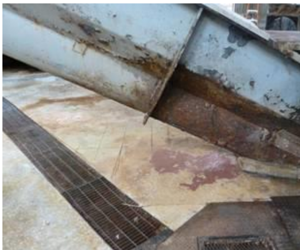
Image 2-4 Leaking Raw Material Trough Image
