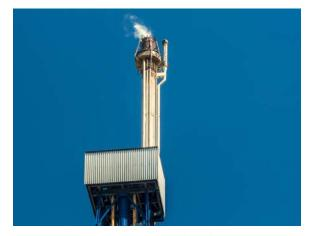
(Image Courtesy: <u>Blackridge</u>) **Figure 2-9. Elevated Flare**
