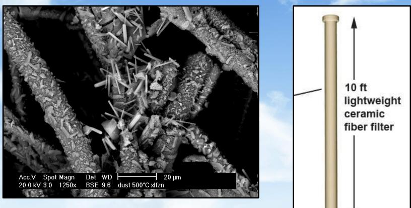
Nano-bits of NOx catalyst are embedded within the fibers and on the fibers
