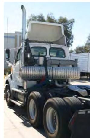
Figure 2: SCCRT Typical System Installation
