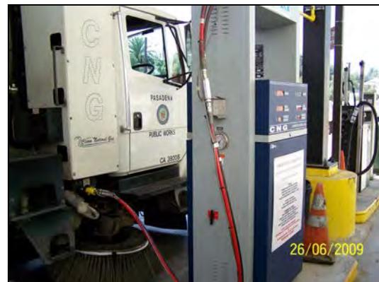
**Figure 3: City CNG Street Sweeper at Fast-fill Dispenser**
