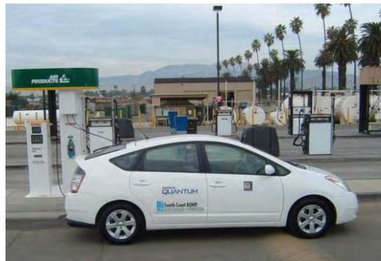
Figure 1: 2008 Toyota Prius Converted to Operate on Hydrogen Fuel
