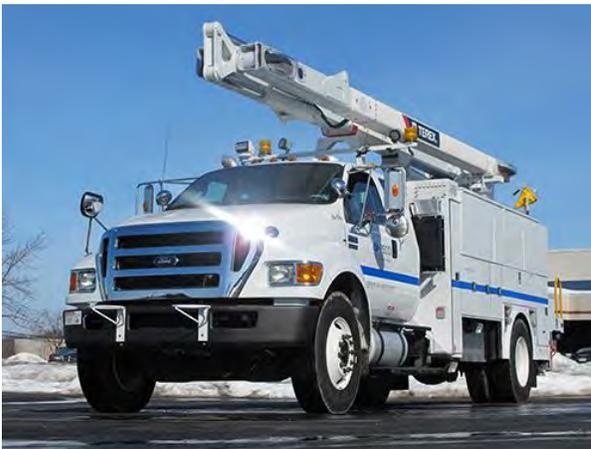
**Figure 7: Class 7 Bucket Truck Equipped with Odyne Plug-In Hybrid Drive System**
