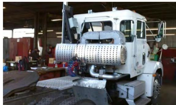
Figure 2: SCRT Typical System Installation
