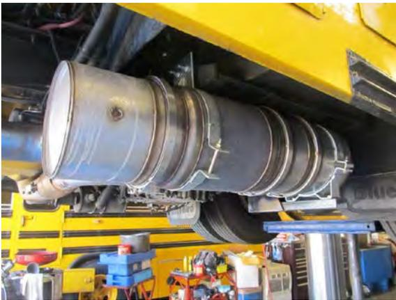
Figure 2: Donaldson LNF installed on Bus 55
