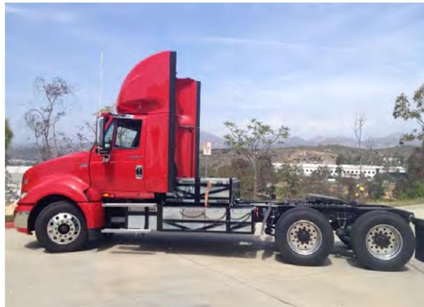
**Figure 6: TransPower Electric Drayage Truck**
