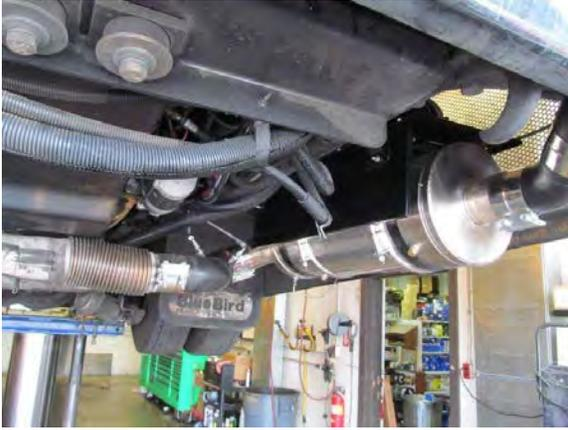
Figure 1: ESW Thermacat installed on Bus 62
