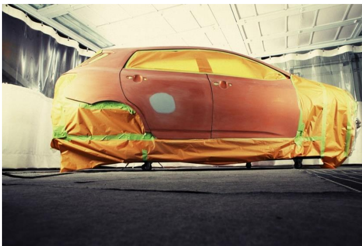
Figure 5-1. Auto body repair shop painting a motor vehicle
