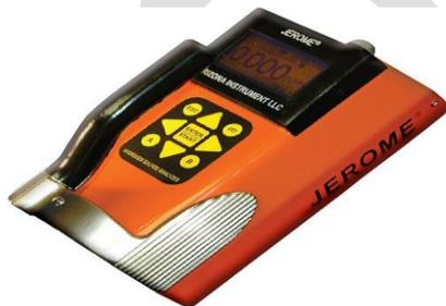
*H<sub>2</sub>S Analyzers (Jerome Meters):* Inspectors can use this handheld instrument to measure hydrogen sulfide gas levels in the air. This information can be used to identify a potential source of rotten egg type odors.
