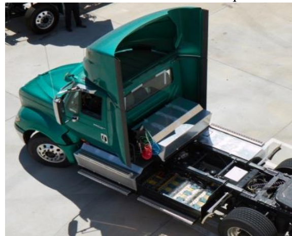
Figure 41: New ESS - 5 large modules (300 Ah cells) mounted on frame rails & behind cab of EDD-2
