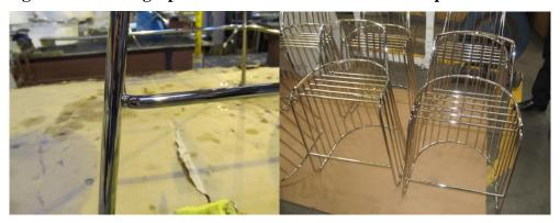
Figure 1-8: Photographs of Trivalent Chromium Electroplated Products
