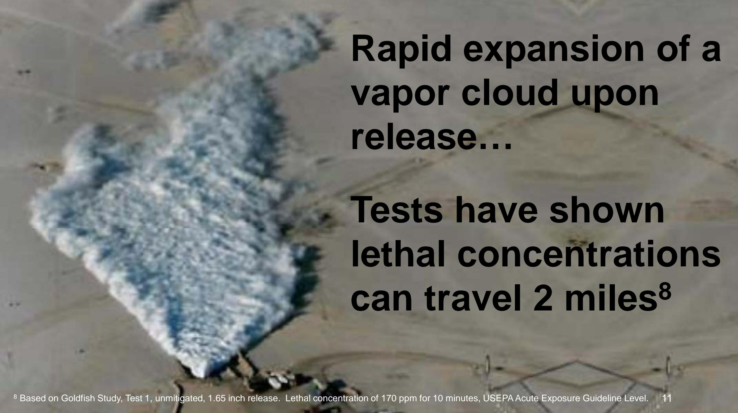
An aerial photograph showing a large, billowing white vapor cloud expanding from a source on the ground. The cloud is dense and has a textured, almost cauliflower-like appearance. It is situated in an open, flat area, possibly a field or a large parking lot, with some faint lines visible on the ground. The background is a light, hazy sky.
