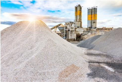
Rock and aggregate (gravel) plants supply sand and various-sized aggregates for construction and paving industries. Aggregates are processed by separating out various-sized pieces of gravel through different sized screens. Oversized aggregates can be crushed into smaller pieces. Dust is created as rocks are crushed and the dry surfaces are exposed, especially as the rocks are more finely crushed.
