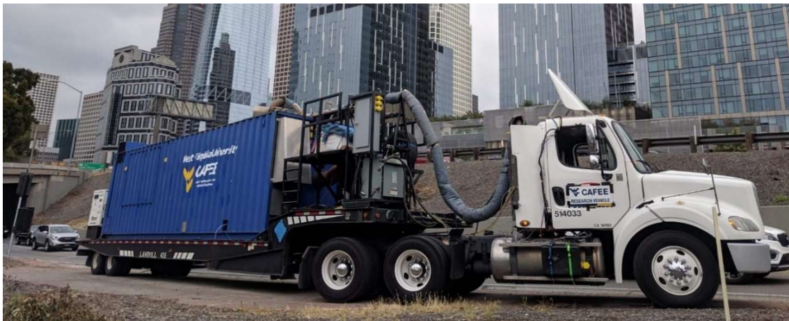
Figure 6: Real-World In-Use Emissions Testing with Lab-Grade Equipment
