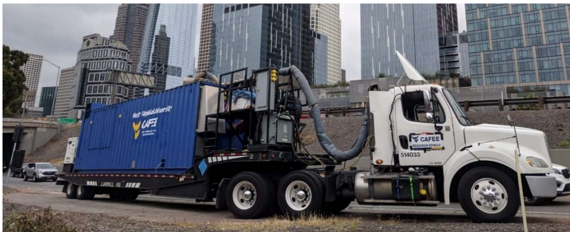
Figure 6: Real-World In-Use Emissions Testing with Lab-Grade Equipment
