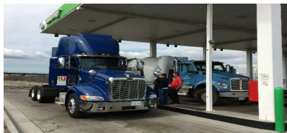
Figure 3: Pac 9 Class 8 with ISX12N Refueling with CNG
