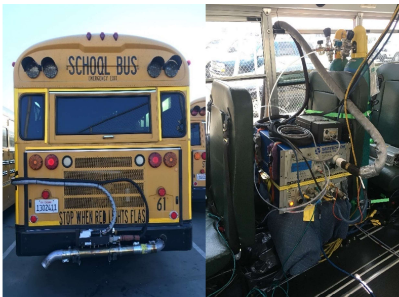
Figure 4: PEMS Equipment Install on School Bus
