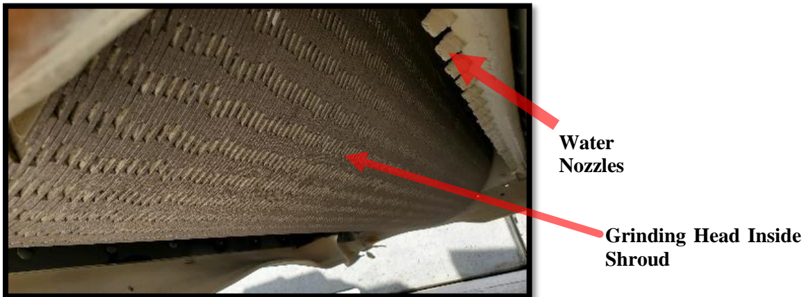
Fig. 2-5: Water Nozzles on Texture Planer
