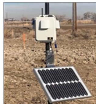
**Figure 2.6 – Example of Area Monitored with Gas Sensor**
