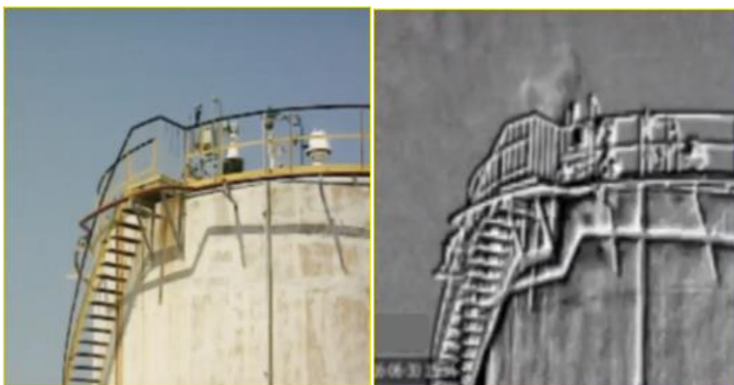
Figure 1-2 View with Naked Eye Compared to View with an OGI Camera
