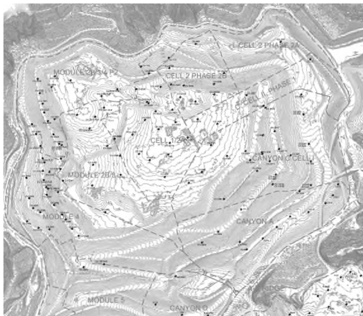
Figure 16. Map of vertical landfill gas wells installed at the Landfill as of December 6, 2023.
