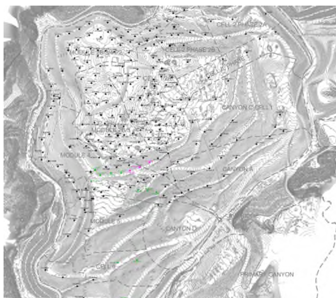
Figure 17. Map of vertical landfill gas wells installed at the Landfill as of October 31, 2024. The green wells are those proposed and in the process of being installed. Chiquita installed over 220 vertical wells between December 6, 2023 and October 31, 2024.
