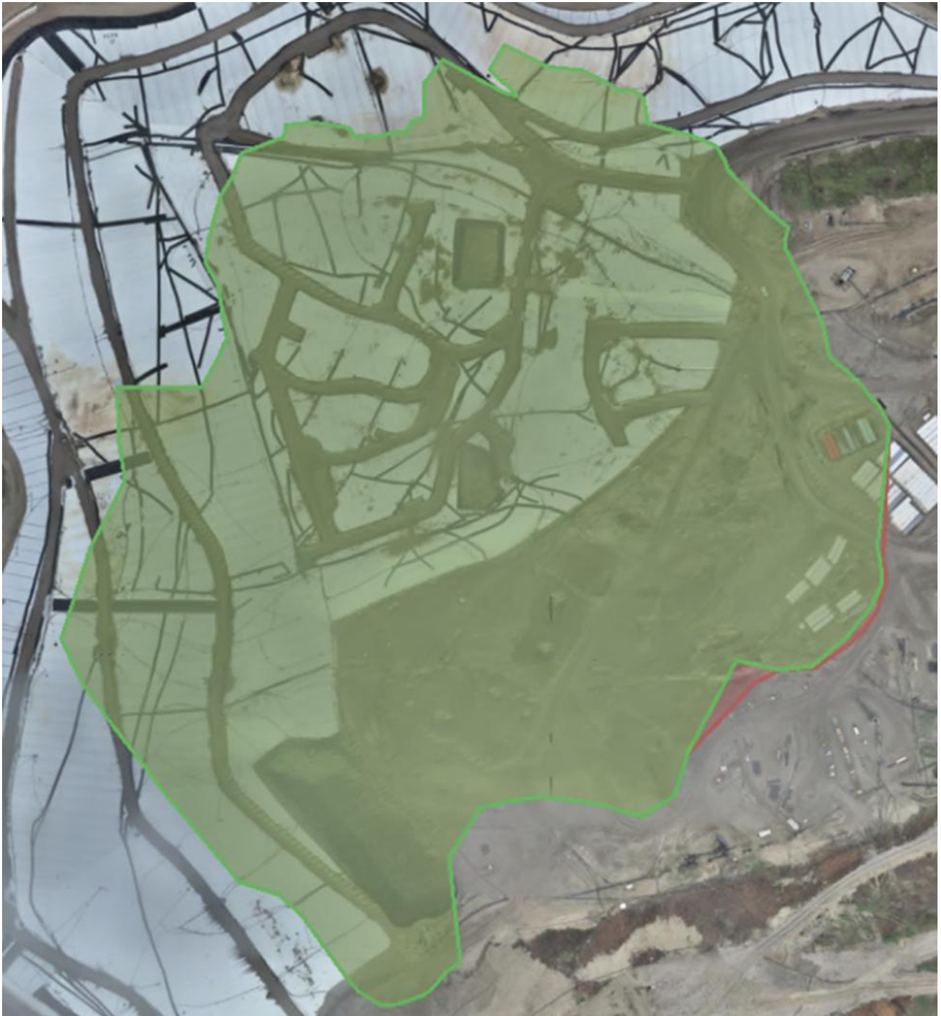
Figure 7. CCL settlement map showing the settlement area growth between 2/26/25 (in green) and 3/11/25 (in red). These polygons show the areas that have settled more than 5 feet. (Source: Bi-weekly Cover Reports by CCL).
