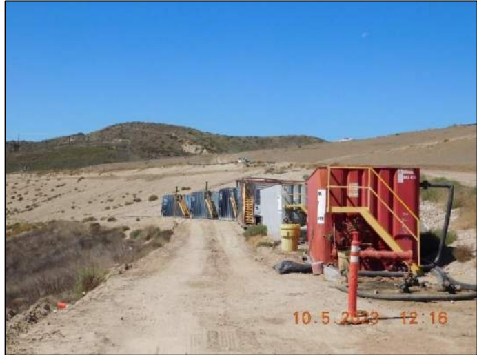
Figure 6 - Baker Tanks for temporary leachate storage.
