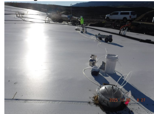
Photo 2.1 Flux Chamber on Membrane Covering Portion of Landfill.
