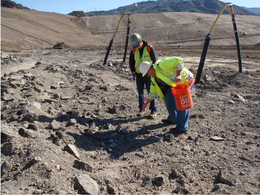
Photo 5.1 Typical Field Screening to Determine Flux Chamber Sampling Locations.
