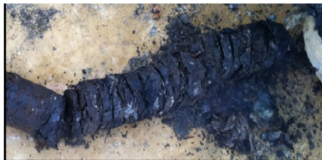
Fig. 9. Core sample of MSW from ETLF site showing similar char formation to inert lab tests.
