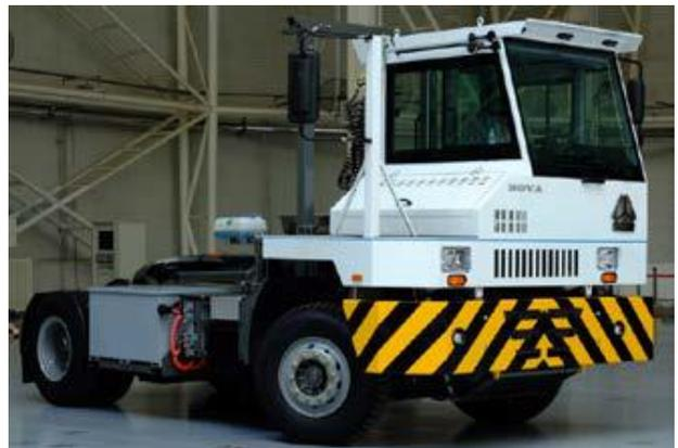
**Figure 10: CNHTC/LOOP Energy Fuel Cell Yard Truck**
