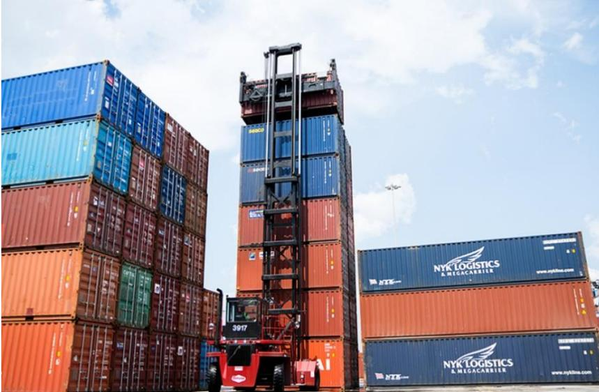
Figure 11: Battery-Electric Top Handler in Service
