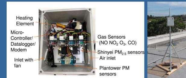
Figure 4. a) Community monitor schematic b) Outdoor Deployment
