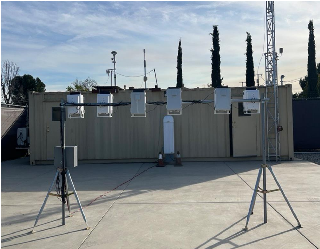
Air sensors undergoing calibration for the Pacoima community monitoring project
