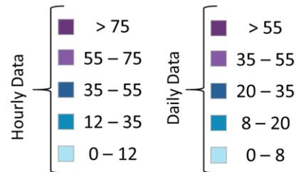
Throughout the DataViewer the above color scale is used to indicate different PM<sub>2.5</sub> levels.
