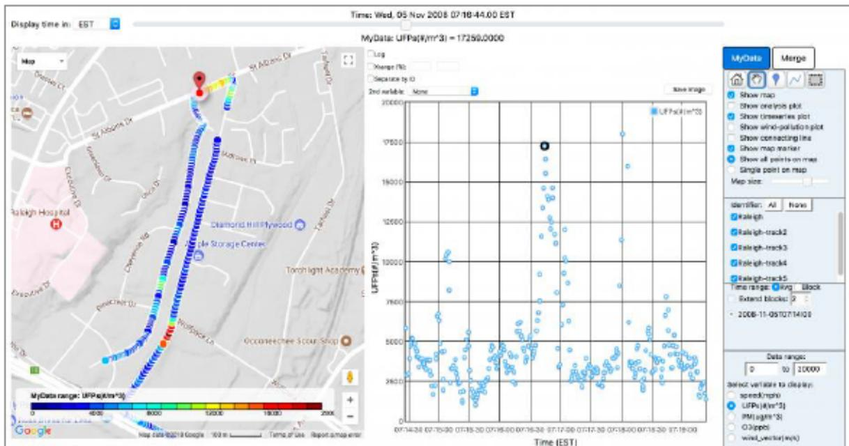
RETIGO Screenshot (source: AQ-SPEC, example of sensor network data with added analysis on the right illustrating pollutant levels in relation to the road highlighted in purple; in this example pollutant levels seem to be higher closer to the road)
