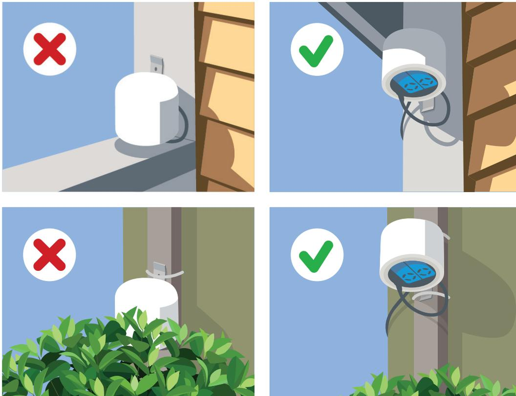
**Figure 4-2.** Proper and improper examples of sensor siting.
