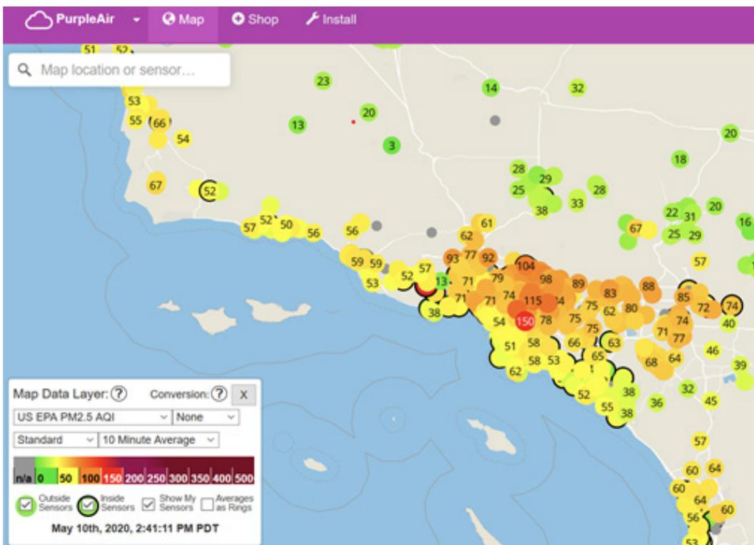
**Figure 4-6.** PurpleAir map showing levels of PM<sub>2.5</sub> using a color gradient and numbers.
