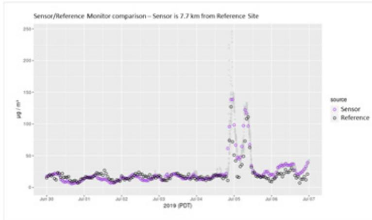
for the entire time period being examined. This period includes the elevated  $\text{PM}_{2.5}$  levels on the 4th of July, and this plot suggests that the elevated  $\text{PM}_{2.5}$  may have been transported from the southwest.
