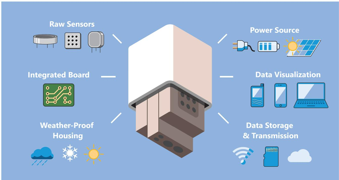
**Figure 2-5.** Basic components of a sensor system.
