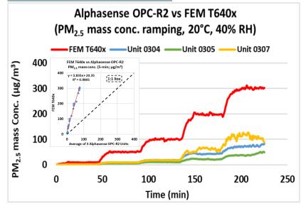
The Alphasense OPC-R2 sensors showed very strong correlations with the corresponding FEM PM<sub>2.5</sub> data ( $R^2 \sim 0.98$ ) at 20 °C and 40% RH.
