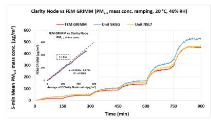
The two Clarity Node sensors showed very strong correlations with the corresponding FEM PM<sub>2.5</sub> data ( $R^2 > 0.99$ ) at 20 °C and 40% RH.
