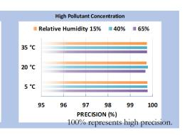
Sensor's ability to generate precise measurements of PM<sub>2.5</sub> concentration at low, medium, and high pollutant levels were evaluated under 9 combinations of T and RH, including extreme weather conditions like cold and dry (5 °C and 15%) cold and humid (5 °C and 65%), hot and humid (35 °C and 65%), or hot and dry (35 °C and 15%).
