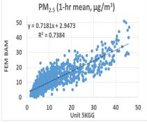
Coefficient of determination (R<sup>2</sup>) quantifies how the three sensors followed the PM<sub>2.5</sub> concentration change by reference instruments.
