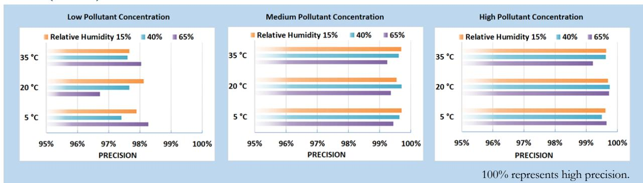
Sensors' ability to generate precise measurements of PM<sub>2.5</sub> concentration at low, medium, and high pollutant levels were evaluated under 9 combinations of T and RH, including extreme weather conditions like cold and dry (5 °C and 15%), cold and humid (5 °C and 65%), hot and humid (35 °C and 65%), or hot and dry (35 °C and 15%).
