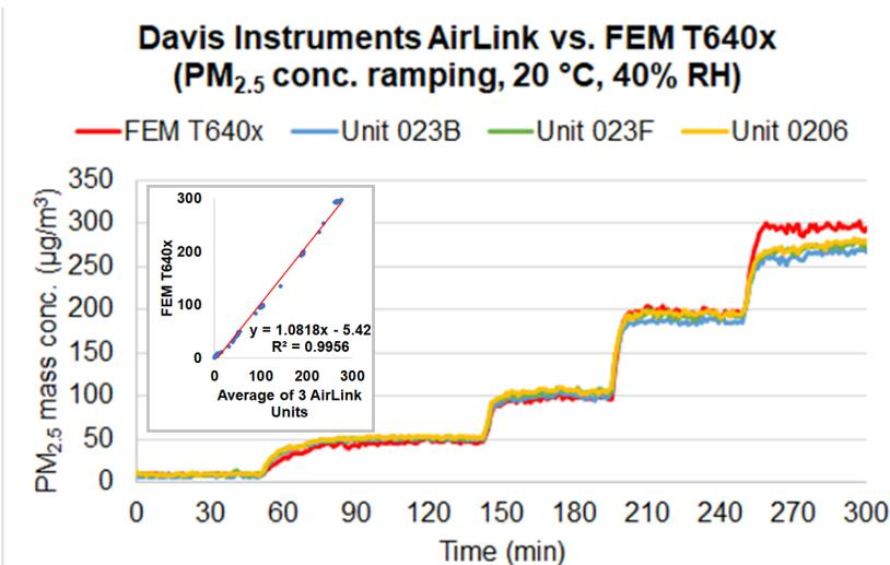
The AirLink sensors showed very strong correlations with the corresponding FEM PM<sub>2.5</sub> data ( $R^2 > 0.99$ ) at 20 °C and 40% RH.
