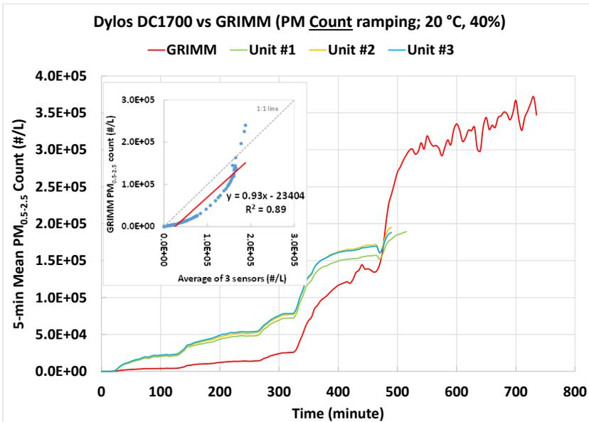
The three Dylos DC1700 sensors showed strong correlations with the corresponding GRIMM PM<sub>0.5-2.5</sub> count data ( $R^2 = 0.89$ ) at 20 °C and 40% RH.
