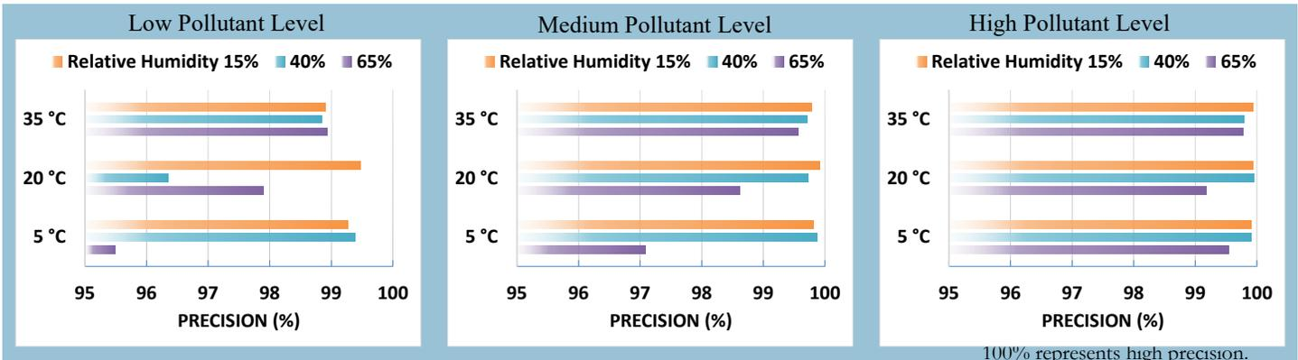
Sensor's ability of generating precise measurements of PM concentration at low, medium, and high pollutant levels were evaluated under 9 combinations of T and RH, including extreme weather conditions like cold and humid (5 °C and 65%), hot and humid (35 °C and 65%), cold and dry (5 °C and 15%), and hot and dry (35 °C and 15%).
