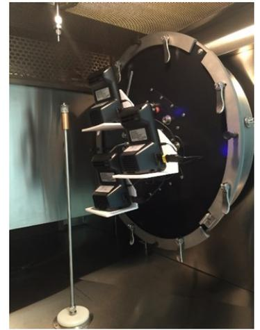
Accuracy was evaluated in a concentration ramping experiment at 20 °C and 40%. The sensor's readings at each ramping steady state were compared to the reference instrument.
