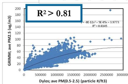
Coefficient of determination ( $R^2$ ) quantifies how the three sensors followed the PM concentration change by GRIMM.
