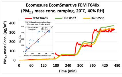
The Ecomesure EcomSmart sensors showed very strong correlations with the corresponding FEM PM<sub>2.5</sub> data ( $R^2 \sim 0.92$ ) at 20 °C and 40% RH.
